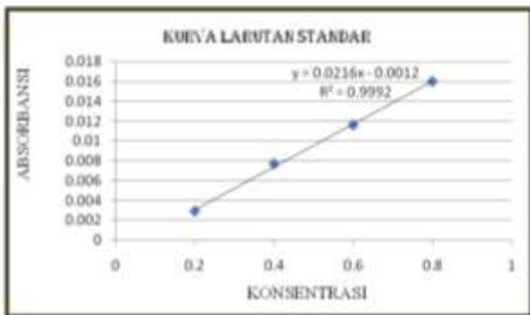
Figure 5. AAS method lead calibration standard curve
